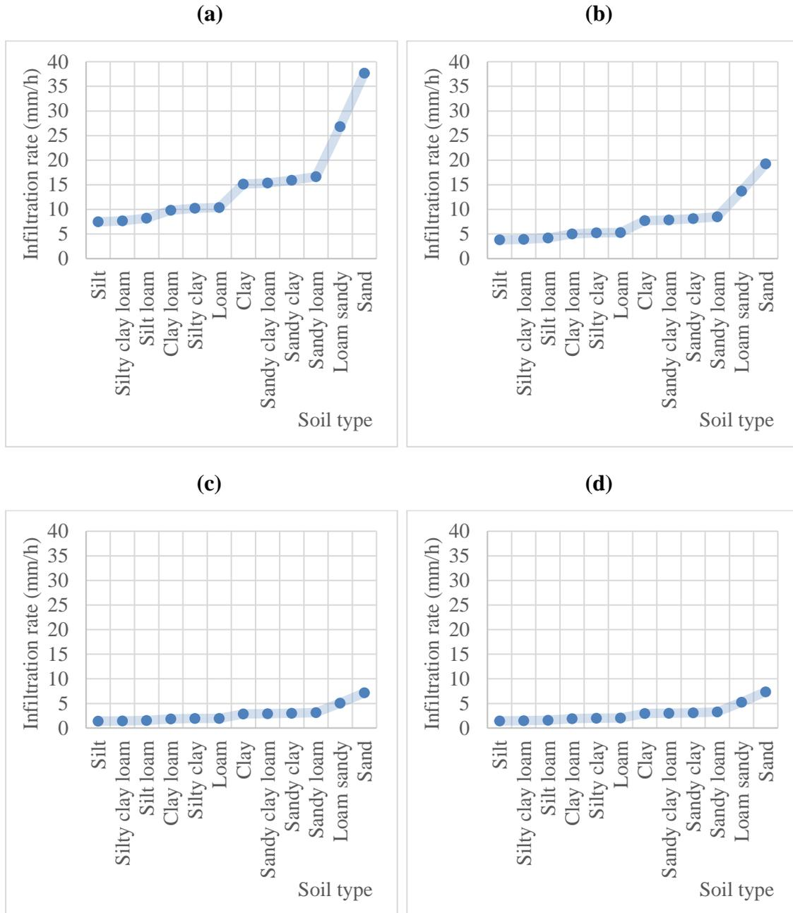
**Figure 6: Infiltration rate of existing soil measured at four test locations on the Birch Lawn at RBGE: (a) Test 1, (b) Test 2, (c) Test 3, and (d) Test 4**
