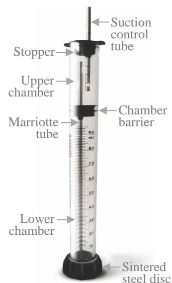
**Figure 4: Mini Disk infiltrometer**
