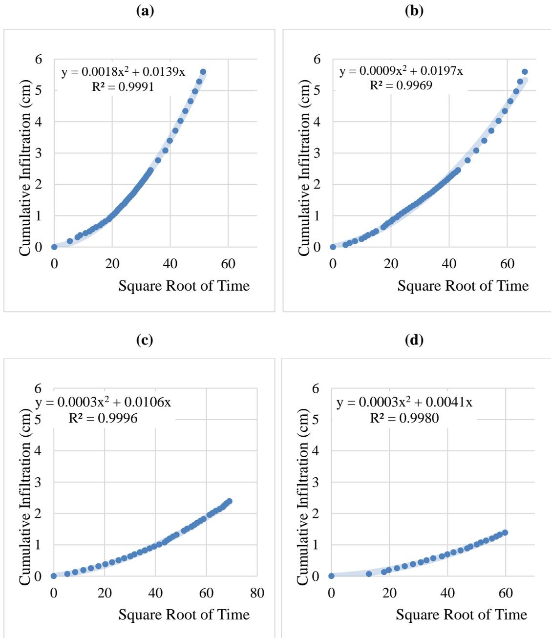
**Figure 5: Cumulative infiltration of existing soil measured at four test locations on the Birch Lawn at RBGE: (a) Test 1, (b) Test 2, (c) Test 3, and (d) Test 4**
